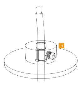
2 COAX must be inserted through the flared end of the strain relief, fender washer must be below this cylinder ring with the strain relief.
