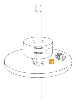
Once at desired length for COAX to be held, simply tighten down hex screw cracking the strain relief so it properly secures the cable.
